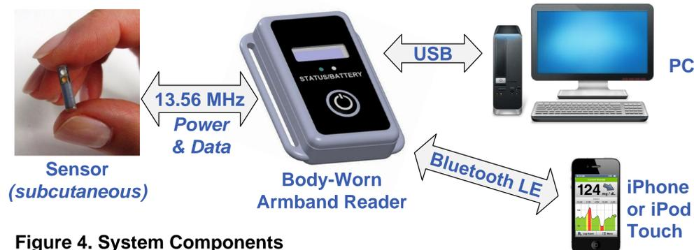
**Figure 4.** System Components
