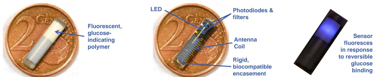
**Figure 1.** Sensor is a miniature fluorometer that detects the fluorescence of an indicator molecule that becomes fluorescent when it binds glucose
