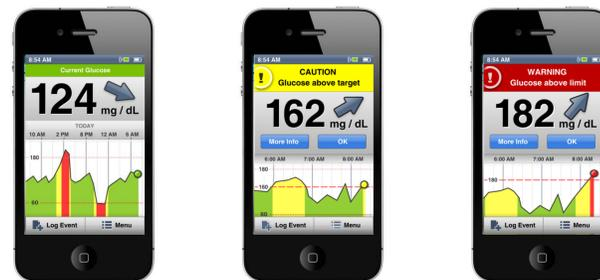
**Figure 6.** Smartphone app displays sensor glucose and issues an alert when a threshold is exceeded
